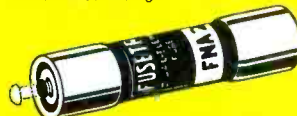
FNA FUSETRON ® dual-element Fuse 13/32 x 1 1/2 in. slow-blowing, Visual-Indicating, Alarm-Activating. (Also useful for protection of small motors, solenoids, transformers in machine tool industry.)
